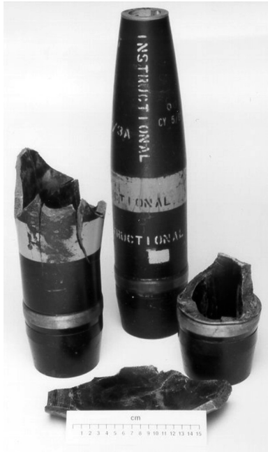
Figure 5. Two 105-mm shells after attack by NM-filled X1E1 either side of an original shell.
